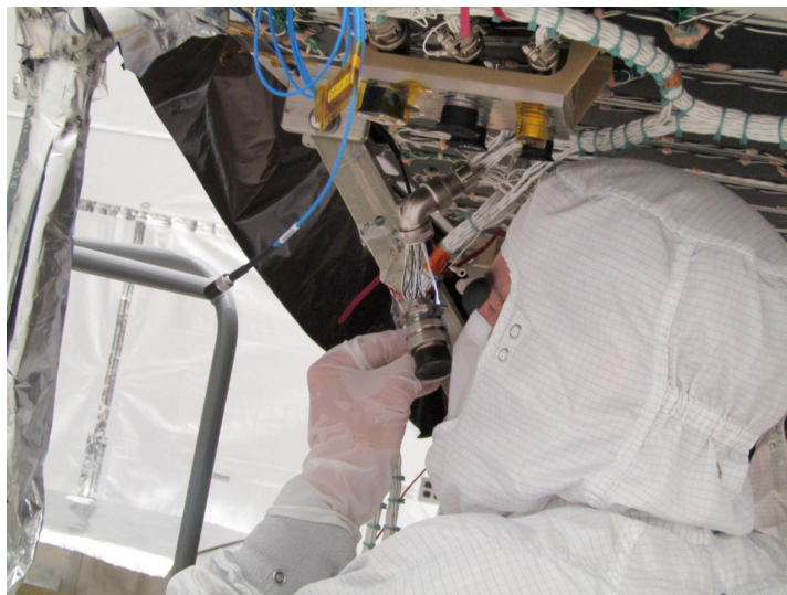
Technician Chris Haag works to repair a connector in the ABI radiator at the L3Harris facility in Rochester, New York. Credit: L3Harris
